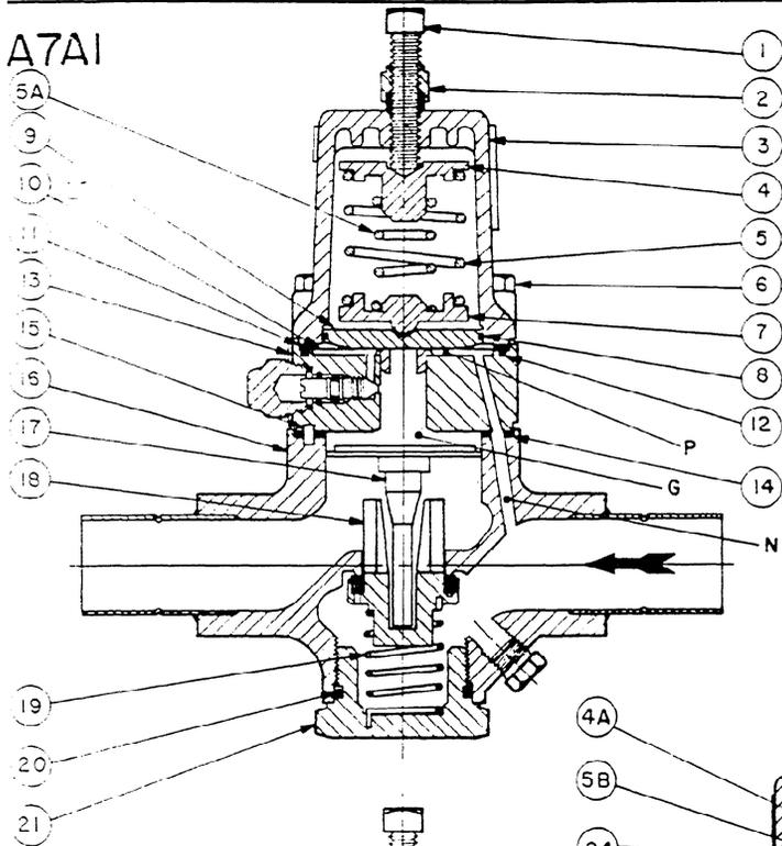
WHEN INSTALLED IN HORIZONTAL LINE, LOCATE ADJUSTING SCREW AT TOP OR SIDE; NOT BELOW CENTERLINE.
