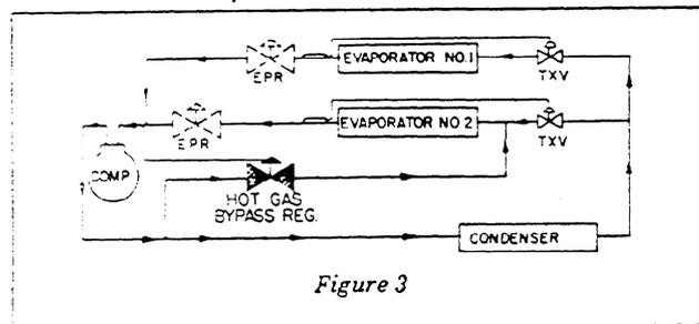
In many applications, an evaporator pressure regulator (EPR) does an excellent job of maintaining evaporator temperature control as loads are reduced. In other cases, the use of an EPR, either preset, compensated by air, by an electric motor, or by a temperature bulb, causes, or may encounter a greatly reduced evaporator load. Below the compressor unloader steps or when
