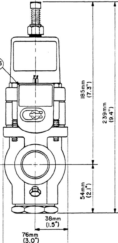
WITH SYSTEM PUMPED DOWN, NO.25 N.P.T. PIPE PLUG CAN BE REMOVED AND OPTIONAL GAUGE OR SCHRADER TYPE GAUGE VALVE INSTALLED FOR INLET PRESSURE READING.
