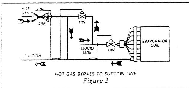
As the load decreases, the suction pressure decreases slightly. The Type A9E regulator, sensing the decreased outlet pressure, opens slightly to meter hot gas through the regulator to the suction. To remove the superheat from the bypassed gas, a liquid injection valve should be installed opposite the A9E regulator.
