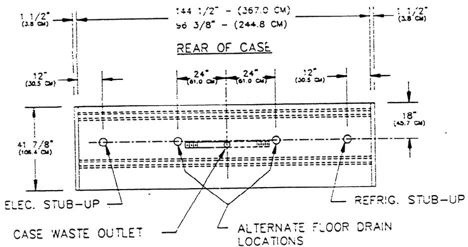
NOTE: DRAIN TRAP AND ELBOW STANDARD
