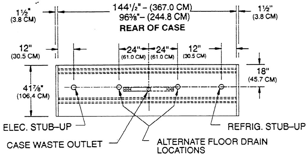
NOTE: DRAIN TRAP AND ELBOW STANDARD
