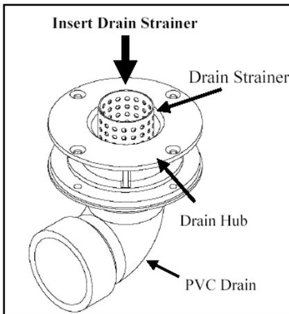
•**Purpose:** Keep debris or any foreign objects from entering the PVC drain which could cause blockage.
