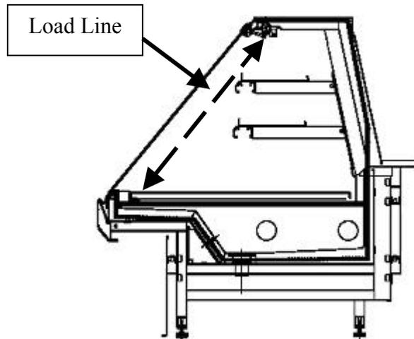
Do not place product in cases until it is at proper operating temperature. Air discharge and return flues must remain open and free of debris or obstruction at all times to provide proper refrigeration and air current performance. Do not allow any product, signs, debris, etc. to block these grilles. Do not use any non-approved shelving, display racks or any accessory that could hamper air current performance.
