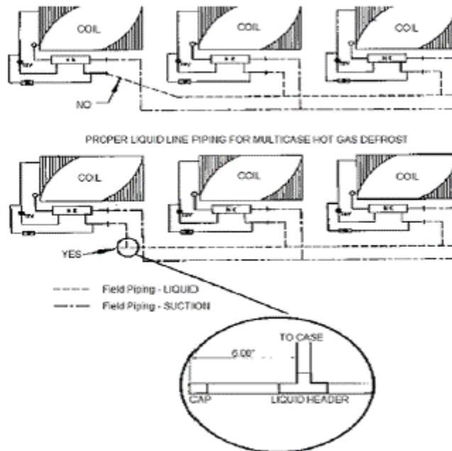
1. Properly sized refrigeration lines are essential to good refrigeration performance. Suction lines are more critical than liquid or discharge lines. Oversized suction lines may prevent good oil return to the compressor. Undersized lines can rob refrigeration capacity and increase operating cost. Consult the technical manual or legend sheet for proper line sizes.
