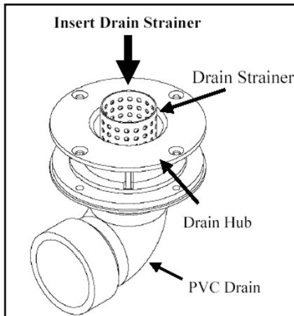
•**Purpose:** Keep debris or any foreign objects from entering the PVC drain which could cause blockage.
