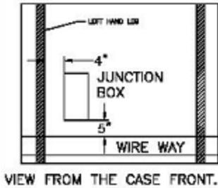
Picture of junction box under the case.
