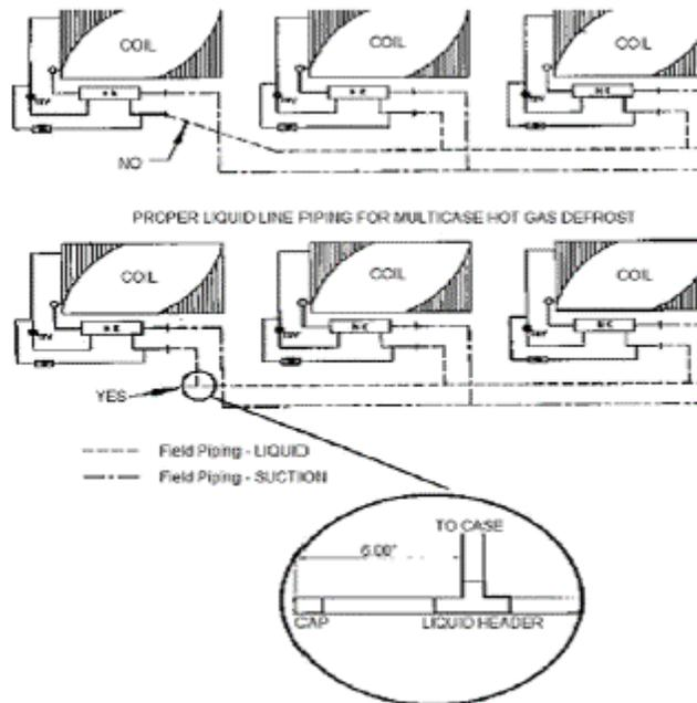
1. Proper size refrigeration lines are essential to good refrigeration performance. Suction lines are more critical than liquid or discharge lines. Oversized suction lines may prevent good oil return to the compressor. Undersized lines can rob refrigeration capacity and increase operating cost. Consult the technical manual or legend sheet for proper line sizes.
