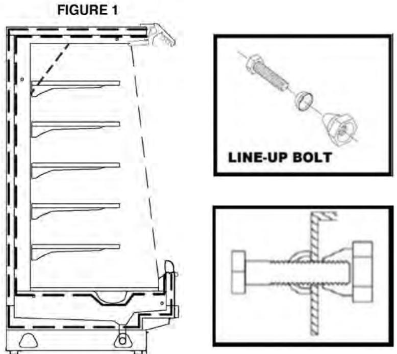
**CASES MUST BE LEVELED FROM FRONT TO BACK AND END-TO-END AND SUPPORTED CONTINUOUSLY AS NEEDED WITH SHIMS.**
