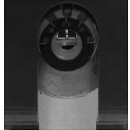
4. Push up on tabs and pull the indicator tab away from the angle dial.
