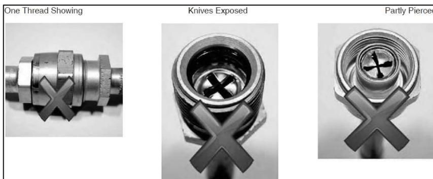
Pictures below show the two parts almost together; the threads are flush. At this point, the main problem will be refrigerant leaks.
