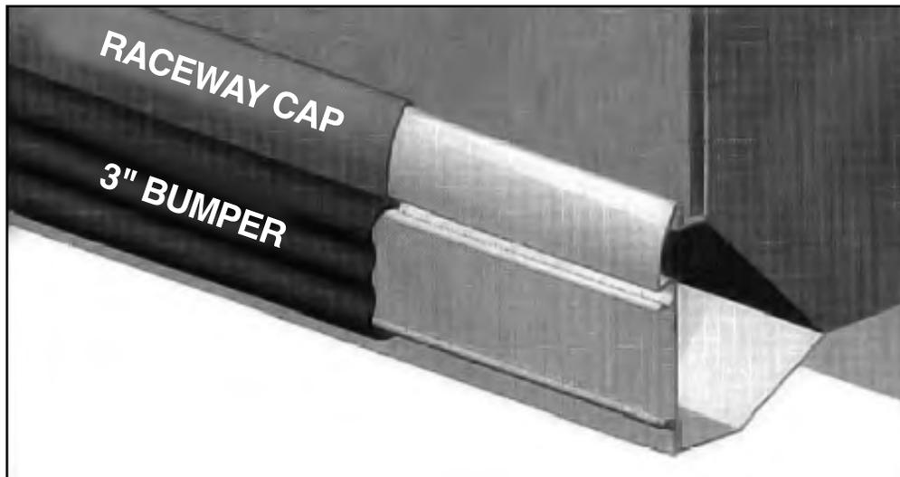
NOTE: The raceway cover parts do not overlap as the rub rail cap parts do.
