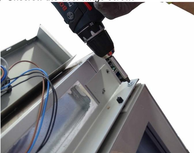
9) Remove the door and the heater wires from the lower support.
