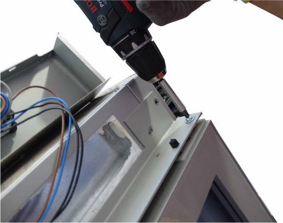
13) Insert and screw the upper door support (use the same screws previously removed).
