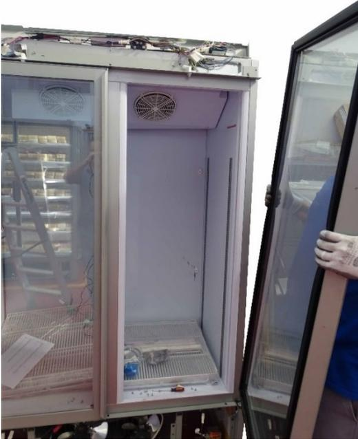
10) Insert the wires into the lower frame (shown as in picture) through the fairlead ring.
